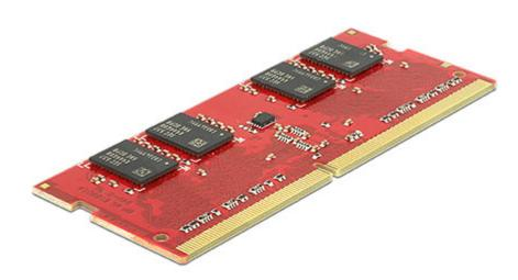
This SO-DIMM is suitable for installation in laptops, industrial PCs and general industrial applications. The memory is ideal for use in harsh environments and has an extended temperature range of -40  $^{\circ}$  C  $_{\sim}$  85  $^{\circ}$  C.
